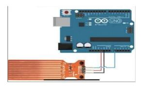
Connect the water level sensor to Arduino as follows:
